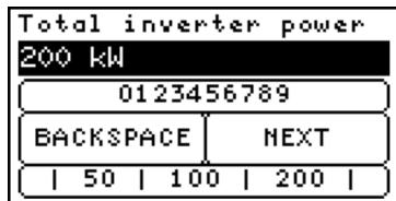
The Embion EMS Controller is able to check the validity of the measured solar radiation, using the actual measured solar radiation and the actual solar power, combining both values using the total PV power configured in the inverter groups. When the generated solar power becomes larger than could be possible with the actual radiation and configured PV power, an error is triggered and the export limit is fixed to 0kW. The error can be recovered in the Zonbalans menu.
