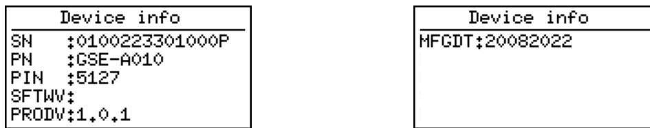
This page shows product information which is identical to the information on the product label. Also current software version is visible in this menu. Also the minimum and maximum internal measured temperatures (during lifetime) are shown here.
