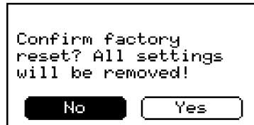
After confirmation, the device will reboot and reset. This will take less than a minute during which nothing is shown on the display and both status LEDs will be off. Once finished, you will be presented with the First Time Use wizard to set up the device again. Note that any license(s) will remain unaffected by the reset and will not be removed during this process.
