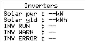
This menu page(s) displays the current status for each inverter. The displayed name of the inverter is the name of the group where it's in, combined with the inverter address. For
