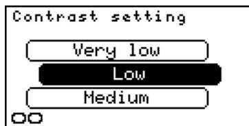
Configures the display's contrast. By hovering over the options, the display contrast will change to the selected intensity.
