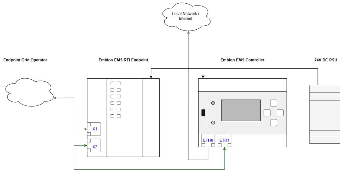
Connect the ETH1 port of the Embion EMS Controller to the X2 port of the Embion EMS RTI Endpoint using the provided, green cable. The ETH0 port of the Embion EMS Controller can be used regularly.
